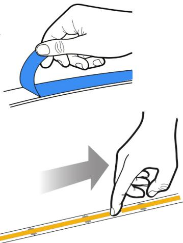
2. Press LED tape firmly onto clean smooth surface that adsorbs heat, such as metal or glass. Start at one end and gradually move along surface, making sure tape is smooth and not creased
