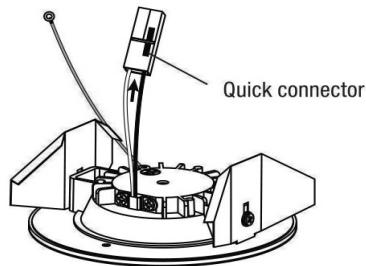
4. Connect the ground wire (yellow-green) by securing the terminal ring to the recessed housing using the provided self tapping screw. Use 1/8" drill bit to drill hole on the recessed housing. Plug in the male and female parts of the connector. Squeeze the bufferfy clips and install the luminaire in recessed housing
