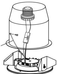
5. Center the luminaire in recessed housing. Install the trim ring by placing the metal size towards the luminaire. The magnets on the luminaire will secure the trim ring in place.
